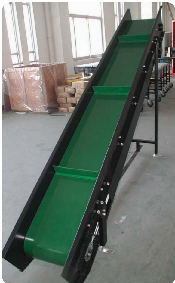
Incline Belt Conveyors CPR001
